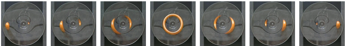
Fig. 2 Snapshots of the images of a billiard ball rolling from left to right behind plexiglass shaped in the form of the foot of a wine glass, illustrating the images of a background star arising from the bending of its light due to the gravitation of an intervening foreground star ( demonstration by Phil Yock, University of Auckland, New Zealand ).
